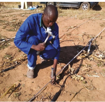
Training in the installation of the ERT sensor arrays at DTC.
