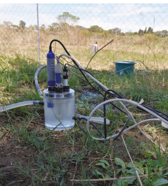
Drilling groundwater boreholes at DTC, Zimbabwe and a flow-through cell in use during groundwater sampling.
