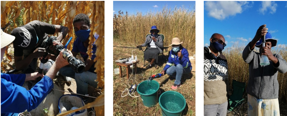
Figure 3 Equipment installation, groundwater discharge rate monitoring sampling and field chemistry analysis during the Zimbabwe pumping test.
