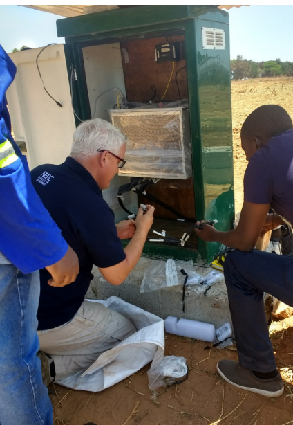
Figure 2 Monitoring equipment installation at Liempe Farm near Lusaka. The PRIME monitoring instrument is being connected to sensor arrays that have been installed within the CA experimental plots.
