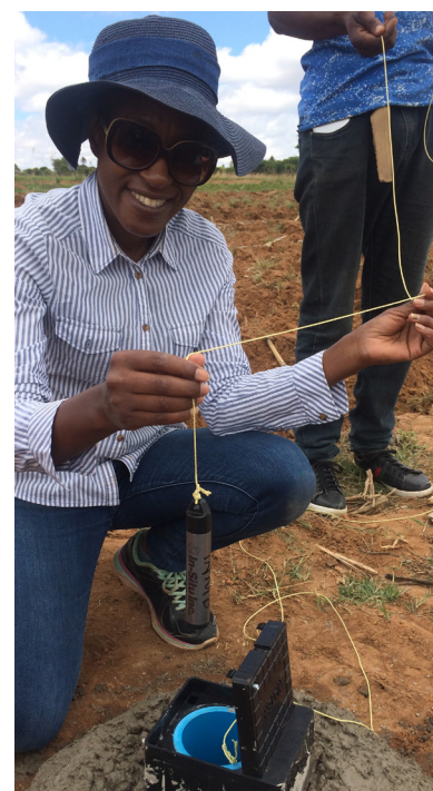
Figure 3 Installation of monitoring equipment at Domboshava Training Centre near Harare. The WIN-SITU data loggers are recording water level fluctuations in the borehole at 30-minute intervals throughout the lifetime of the project.
