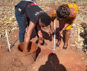
Figure 2a Training in installation of ERT sensor arrays and connecting the sensor arrays to the monitoring equipment at Chitedze.
