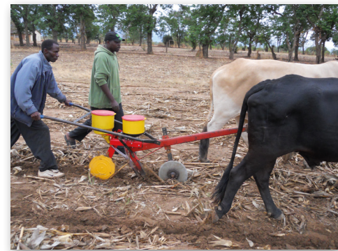
Mechanising direct seeding with animal power.
